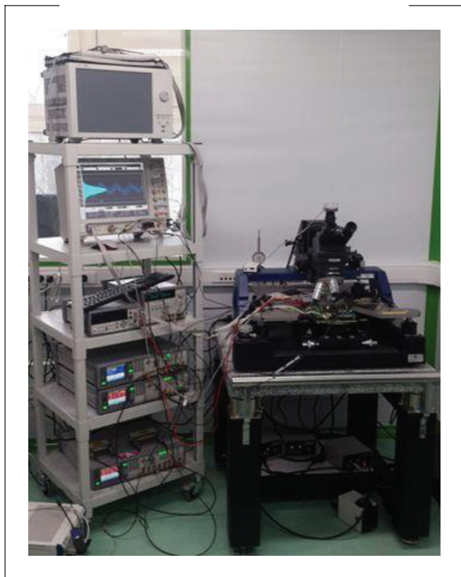
Figure 2 Measuring equipment and probe station
